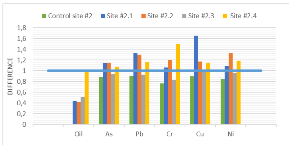
Figure 3. Changes in the content of metals and metalloids due to treatment
